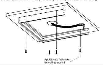
5.Put the wire conduit hose as close as possible to the surface mount opening before placing/inserting the luminaire into it partially. Make all electrical connections according to local code and make sure wire conduit hose is long enough for wiring connection inch
