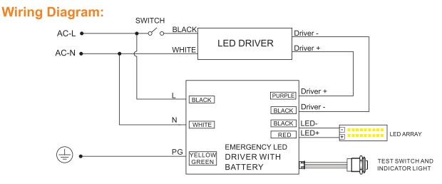
1.DO NOT MATE CONNECTOR UNTIL INSTALLATION IS COMPLETE AND AC POWER IS SUPPLIED.
