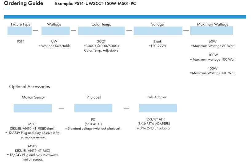
Note: 1. For photocell and motion sensor, special factory installation is needed. Contact factory for availability and lead time.
