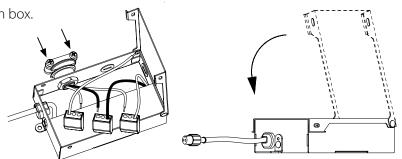
5 Connect light engine. Be sure to properly align connectors and fully screw down connector cover.
