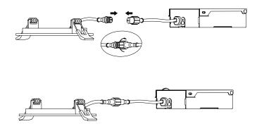
6 Place driver box into ceiling. (Optional: Mount using mounting tabs and screws)
