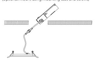
Push up spring-arms on side of fixture, lift into ceiling, and release spring-arms.
