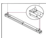
**Step1:**Attach aircraft cable to each hook and insert hooks into the mounting holes.
