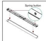
**Step1:** Install appropriate anchors into the ceiling or wall, if needed. Pinch spring buttons to remove the lens.
