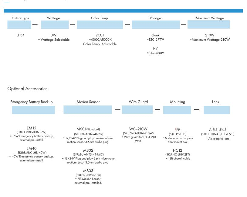
Note: 1. Surface mount/pendant mount is not support when the fixtures installed the emergency battery backup.
