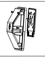
3) .After installation, daub the gap between installation board and wall by waterproof glue to avoid leaking, Hang the rope to cover of driver to avoid falling. And connect AC wire.
