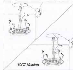
3. Push all connected wires (also 3CCT button and connected wire for 3CCT version) into the housing with caution. Press the friction blade to insert the luminaire.
