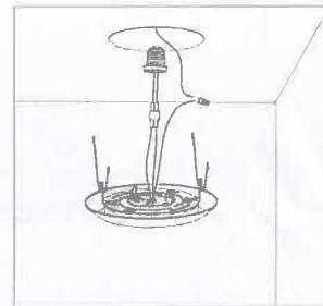
2. Screw E26 socket adapter into socket in the housing. Connect the wires by using the wires nuts
