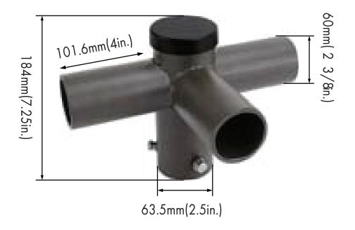
Triple 90' Horizontal Tenon Adaptor Part number: PKBRK-TN3TAP Finish: Dark Bronze USE: The Bracket is designed to mount over 2-3/8" (60mm) O.D. vertical tenon. Three fixtures can be mounted to the Round External Mount Horizontal Tenon and adjusted horizontally
