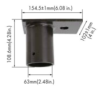
Pole Bracket accessories-Tenon & Yoke Adaptor NO. SP-TR-D Finish: Dark Bronze USE: The 2-3/8" OD Tenon Mount Adaptor for Yoke Fixtures is designed to mount light ÿxtures that are equipped with a yoke mount onto a 2-3/8" OD tenon. It may be utilized with the Mester Flood Light Series of light ÿxtures.
