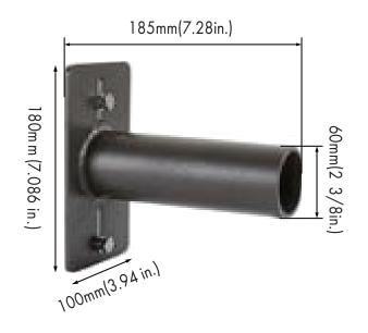
Part number: PKBRK-SPRAP Finish: Dark Bronze USE:2-3/8" OD Horizontal Tenon Mid-Pole Bracket is designed to mount light fixture that is equipped with a adjustable slipfitter onto a 2-3/8" OD horizontal tenon
