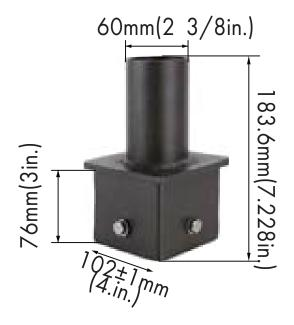
4" Square Pole Mount with 2-3/8" O.D. Tenon Part number: PKBRK-4SQAP Finish: Dark Bronze USE: For use with square, non-tapered steel and aluminum poles. Furnished with four 5/16" hex head stainless-steel bolts. Vertical tenon measures 2-3/8" O.D., and is made of steel tubing. Fixtures mounted to this bracket can be adjusted both vertically and horizontally.
