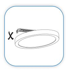
DON'T REMOVE THE FIXTURE FROM ANY ONE SIDE OF THE SELF-LOCK MOUNTING STRAP. THIS MAY CAUSE DAMAGE TO THE FIXTURE
