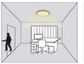
The fixture will remain in standby mode when no motion is detected.
