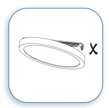
DON'T REMOVE THE FIXTURE FROM ANY ONE SIDE OF THE SELF-LOCK MOUNTING STRAP. THIS MAY CAUSE DAMAGE TO THE FIXTURE
