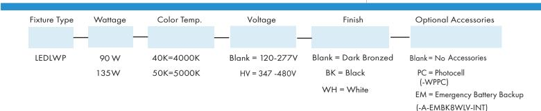
Note: The emergency battery backup only compatible with 90W
