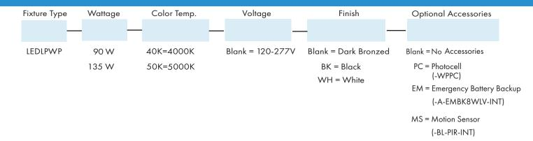
Note: The emergency battery backup only compatible with 90W
