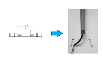
3. Join the light to hazardous location cable pipe, connect the AC the Live wire, Null wire and grounding wire, close the power enclosure. Fix the light on the ceiling or wall.
