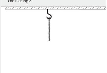
4. Hang the fixture to the hook as above, connect the AC cable, Black cable joins to L, white cable joins to N, green cable joins to grounding.
