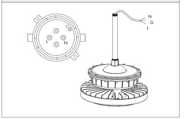
3. Install the installation box to the wall or ceiling as Flg.2. Tighten the pole to the box, and adjust the chain of balance.
