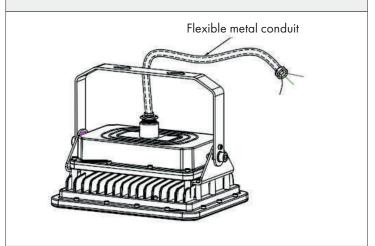
4. Connect the AC cable,Black cable joins to L,white cable joins to N, green cable joins to grounding.
