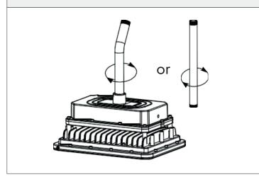
2. ConnecttheACcable toinstallationbox,Black cablejoins to L white cable joins to N green cable joins to grounding.
