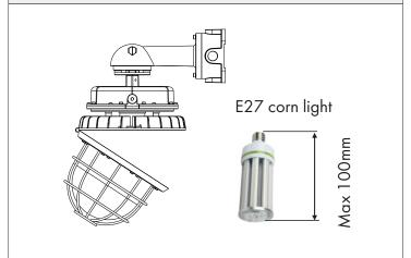
3. Tighten M5 screws via 4# allen key, double check the gap is less than 0.5mm.
