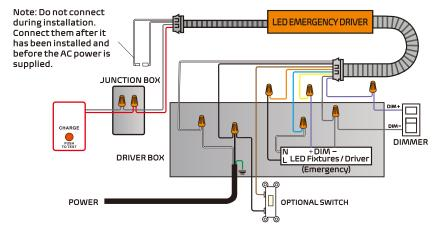
2. Wiring If Power Of Luminaire ≤power Of Led Emergency Driver.
