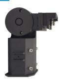
**Slipfitter Mount** - An optional cast aluminum arm adapter secures fixture head to nominal -3/8" O.D. horizontal steel tenon arm.
