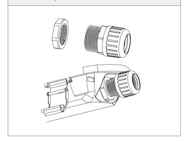
Feed the wires from the electrical source through the cord grip and into the fixture body.
