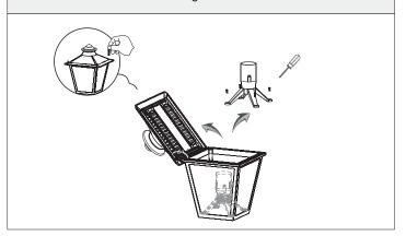
2. After removing the bracket, fix the power wire with a wire clamp, and fix the wire clamp with screws.
