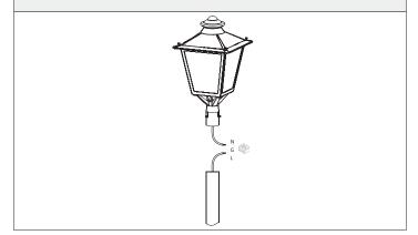
5. Install the fixture into the pole and use a hexagon wrench to tighten the three fixing screws.
