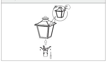
4. Connect the input wire to the pole, and connect the reserved wire with the terminal.
