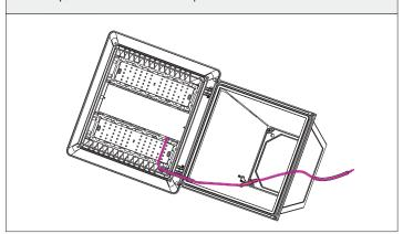
3. Install the bracket to the housing, and lock the bracket with the fixing screws removed in the first step.
