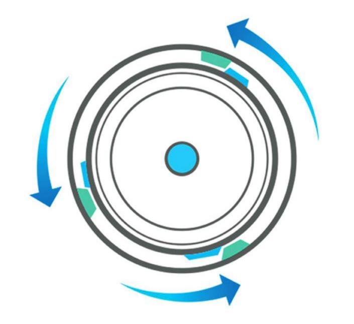
The Twist & Lock feature allows for easy, tool-free installations and seamless integration of multiple trims.
