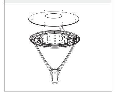
4. Unscrew the waterproof plug pull the fixture lead, center luminaire on tenon and tighten supplied set screws to securely mount luminaire to tenon and pull the fixture lead.Remark: 3" tenon(default seting); 2 3/8 pole adapter provided.Connect wires (voltage to black, white to common, green to ground). Once connections are completely made, carefully push all wires down into the junction box and secure it with waterproof plug.
