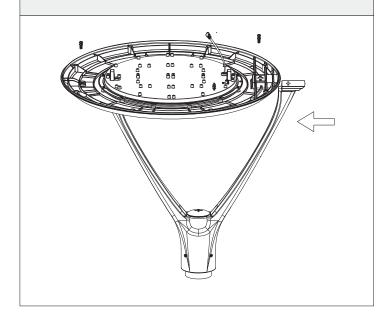
3. Feed supply wire through center of tenon and through center hole in post top arms and make cable joint connector connections with driver; and cover should snap into place according to the arrow; secure top cover with (8) M5X16 screws and make sure (8) rubber cover in the corresponding position.
