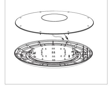
2. Push the Y-pole horizontally along the fixture track groove and secure the fixture and Y-pole with (4) M6X12 set screws.
